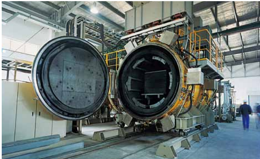
Large Sintering Furnace for Carbon-fiber Insulation (Kureha Chemicals Shanghai Co., Ltd.)
